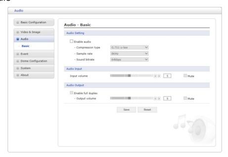
The camera can transmit audio to other clients when using an external microphone and can play audio received from other clients when using an attached speaker. The Setup page has an additional menu item called Audio, which allows different audio configurations, such as full-duplex and simplex.
