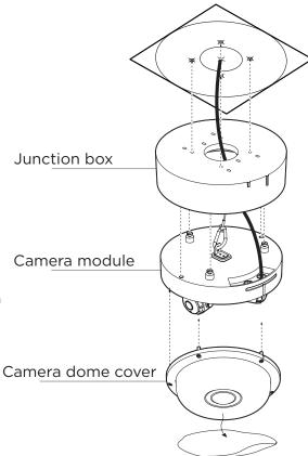
Adjust the camera modules' position and angle and complete the installation by placing the dome cover on the camera. Secure the dome cover to the camera base using the screws included with the camera. See the camera's QSG for more information.
